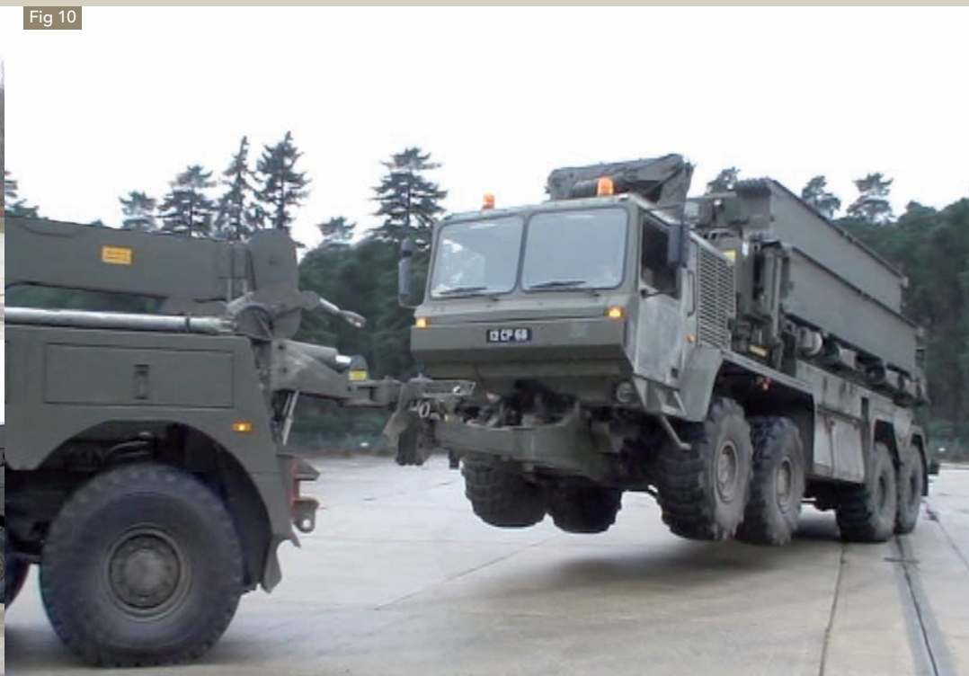
Fig 10 | Front suspend tow. Unipower BR90 using Unibeam attachment.
