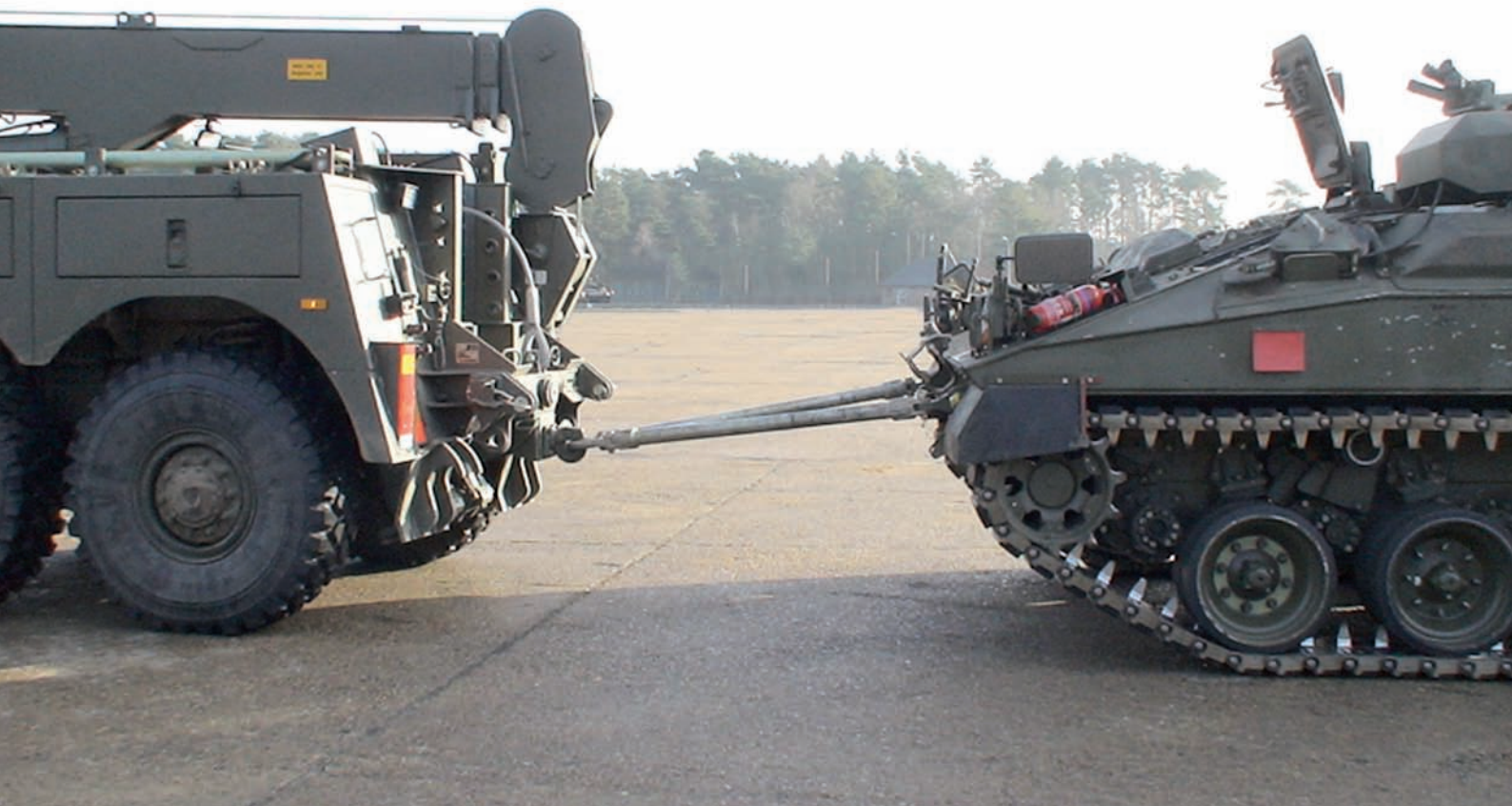
Fig 5 | SuperCompact with 'swing-away' towing pintle deployed. Demonstrated towing Warrior on Hollebone system.
