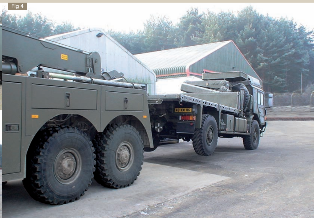
Fig 4 | Rear suspend tow. MAN 6 tonne Cargo during System integration trials.
