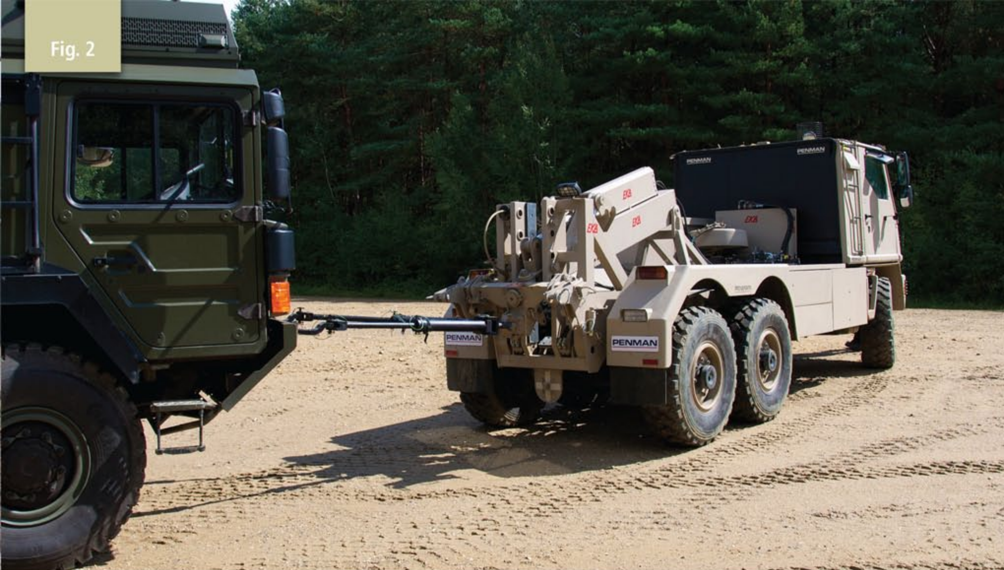
Fig 1: . . . . . Two-part winch recovery pulls up to 16 tonnes are possible, using the innovative ground anchors. Rope runs are arranged at high level to help extract the casualty.
