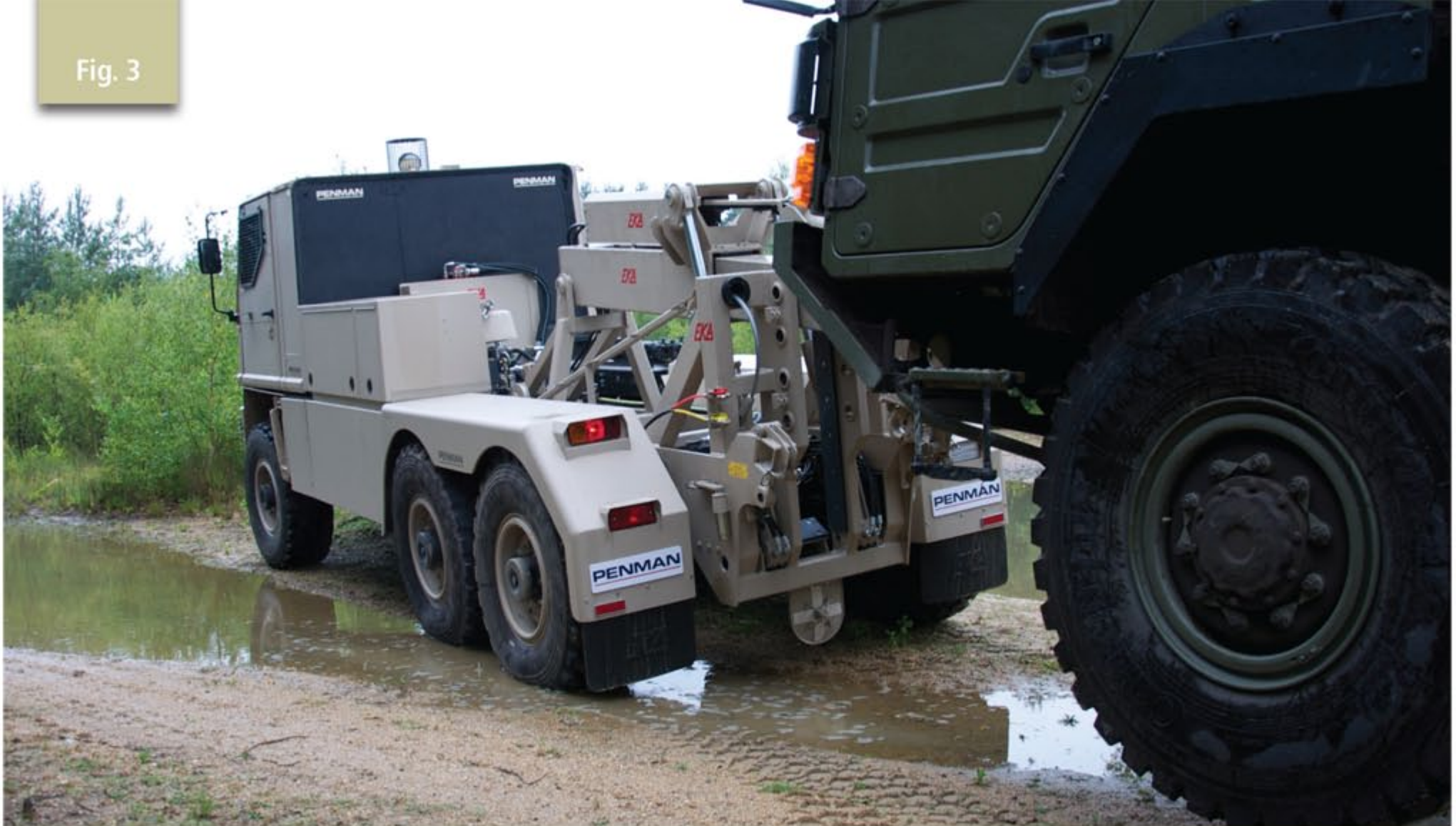
Fig 4: . . . . . The variable-height recovery device can be pinned at four different heights, to ensure that even very small casualties can be safely towed.
