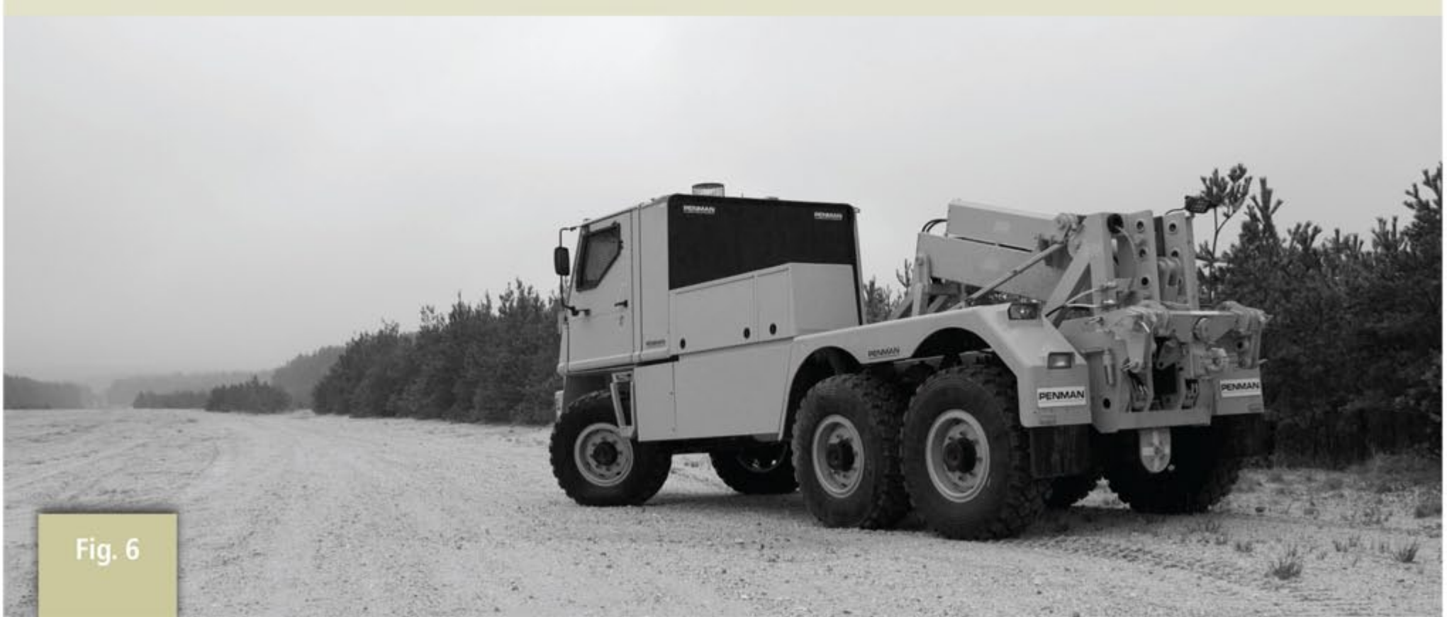
Fig 6: . . . . . Compact weight-conscious recovery equipment design, a host chassis with good mobility, manoeuvrability, and a maximum width of 2.2 metres, make the Lightweight Recovery Vehicle the ideal asset for intimate recovery operations.
